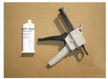
6. To use the cartridge material, an appropriate type and size of the cartridge gun is required.
