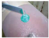
9. The cartridge is now ready for use. When gun is operated, the plunger will dipense Part-A and Part-B material in proportionate amount. The epoxy is mixed in the static mixer and comes out as mixed material. (Note: Each use of the cartridge requires a new static mixer.)
