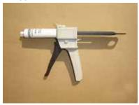
7. Place the product filled cartridge properly into the cartridge gun as shown in this picture. The cartridge must fit properly.
