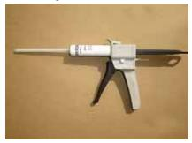
1. The Powercrete® R-65/F1 dual component epoxy cartridge is sealed and has a cap on the end of the nozzle. The cartridge contains both Part A and Part B of the Powercrete® R-65/F1 epoxy, in ratio, for the correct mix when used with the supplied static mixer. At the time of use, the cartridge temperature must be above 20°C (68°F).
