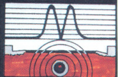
AUDIO RECEIVER TONE AS PIPE IS CROSSED
