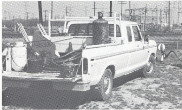
Personnel pick-up truck carries hoses and fittings for installation of Fill-Coat #1. Pick-up truck also carries heating, safety and cleaning equipment.
